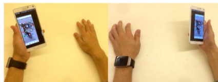
Figure 5: WhichHand makes a Reduced Screen interface automatically adjustable to a user's left or right hand whenever switching hands
